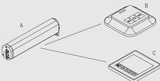
In addition to the fixed wall switch, the 5100T is supplied with a timer unit which allows pre-programmed opening and closing times.
